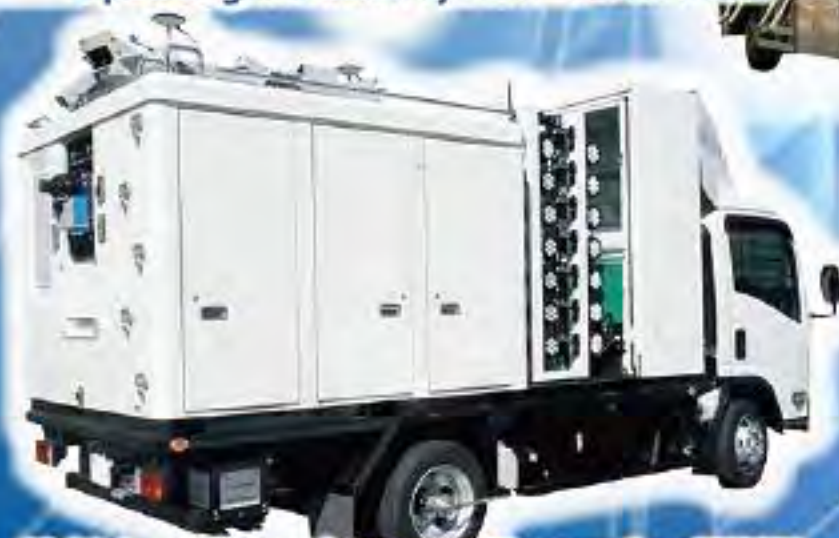
Vehicle dedicated to tunnel inspection MIMM
