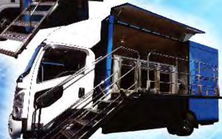
Battery power generation type earthquake experience vehicle 4 t type VE-T4
