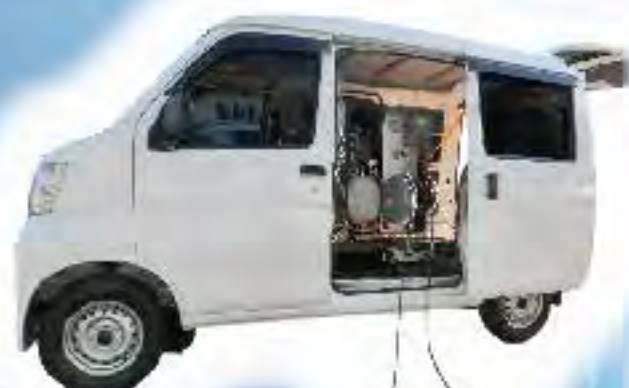
Kei-van equipped with an air compressor & a power generation system "K Den-Maru"
